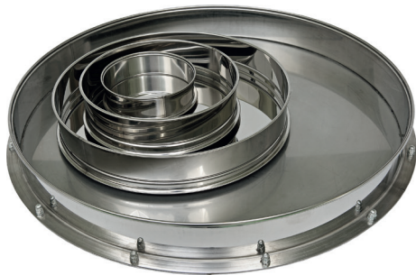
Trays with diameter of 120, 200, 300 and 500 mm
